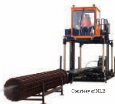
FIGURE 1. Heat-exchanger cleaning programs have become an important part of energy-management systems. Shown here is hydroblasting equipment for cleaning shell-and-tube heat exchangers
