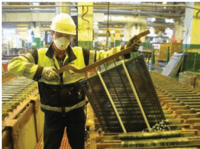
FIGURE 1. Shown here is Outotec's Cu electrowinning (EW) anode. EW plants utilize hundreds to thousands of electrodes to recover high-purity metals
