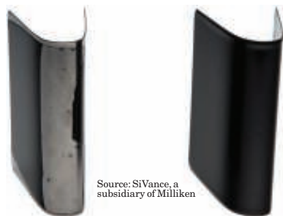
FIGURE 1. SiVance's C1008 is a silicone curative that improves the durable flexibility of epoxy polysiloxane protective topcoats in marine and infrastructure applications
