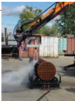
FIGURE 1. Heat-exchanger cleaning programs have become an important part of energy-management systems. Shown here is hydroblasting equipment for cleaning shell-and-tube heat exchangers
